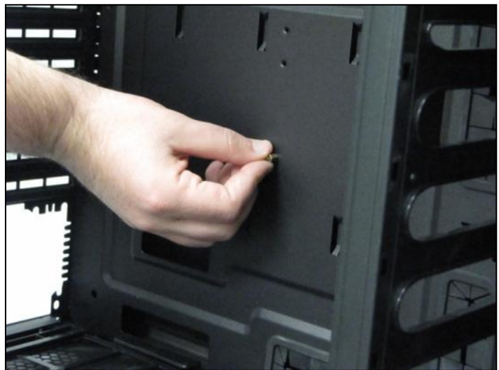
Install the motherboard standoffs by aligning the motherboard with the standoff holes.
