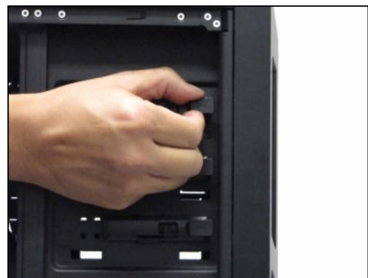
Pull on the tab to adjust drive bay clearance.
