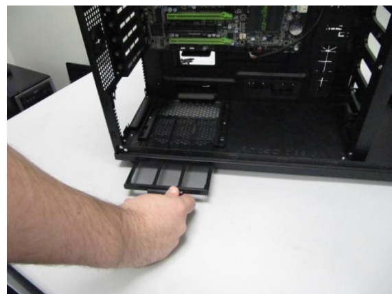
Pull the filter toward you using the tab outside the chassis.
