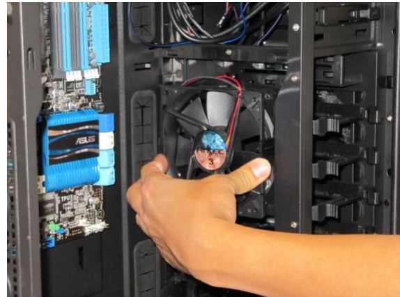
Secure an intake fan into place by aligning it with the pegs that correspond with the fan screw holes.
