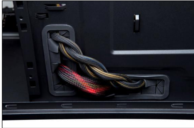
Use the grommet-lined cable routing holes to route PSU cables.
