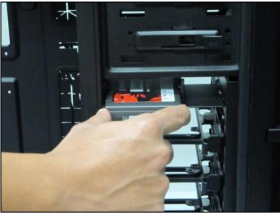
Align your drive's holes with the drive bay holes when sliding it in.
