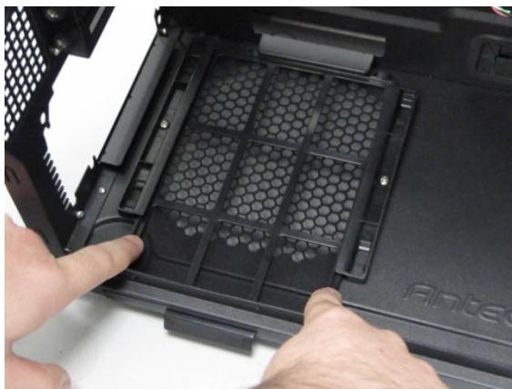
Unlock the filter by pushing down on the filter's ends.
