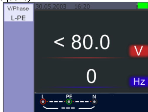
Standby screen for the Voltage and Frequency
