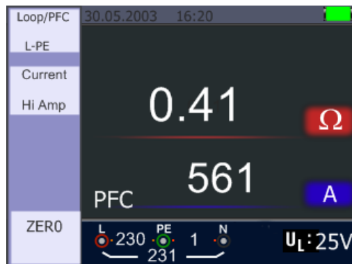
Hi Amp LOOP – Measurement finished
