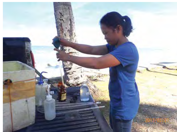
On-site analysis of DO, pH and temperature.
