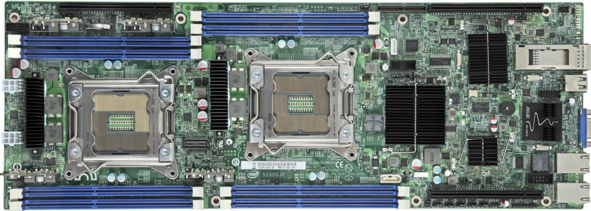
Figure 7. Intel® Server Board S2600JFQ/S2600JFF
