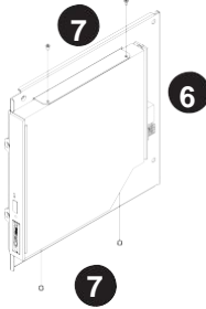
Figure F-4: Installing the Lower Bracket onto the DVD-ROM Drive
