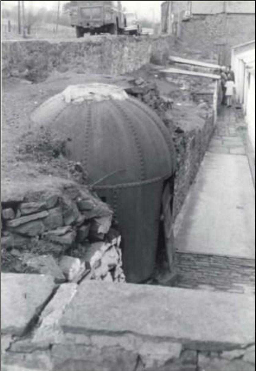
Canal side, an old Beehive air receiver, one of the few remnants of the Gethin Collieries. (Photograph courtesy of The John Owen Collection)
