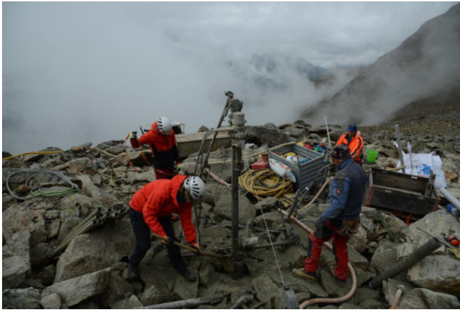
Fig. 57. Borehole drilling in August 2020 on the ice-rich Schafberg rock glacier. Photo: Nora Bühler.
