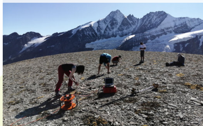
Fig. 2. ERT measurements at Mittlerer Burgstall (2933 m asl) to detect and quantify the distribution of permafrost.
