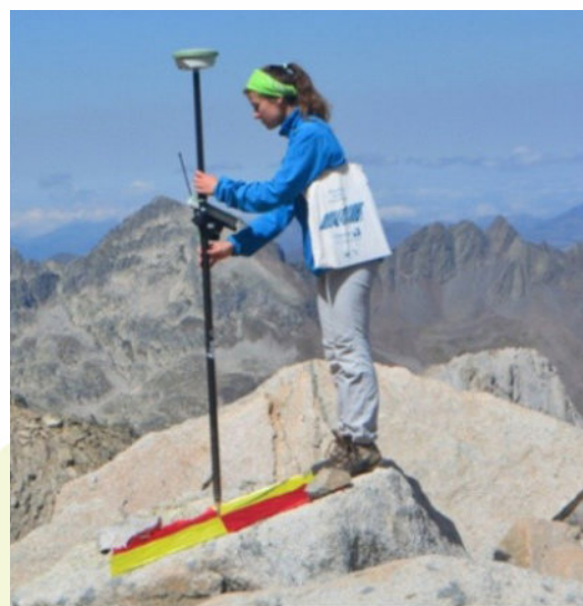
Fig. 53. La Maladeta, Pyrenees. Top: view of La Maladeta rock glacier. Bottom: GPS-RTK measurements.
