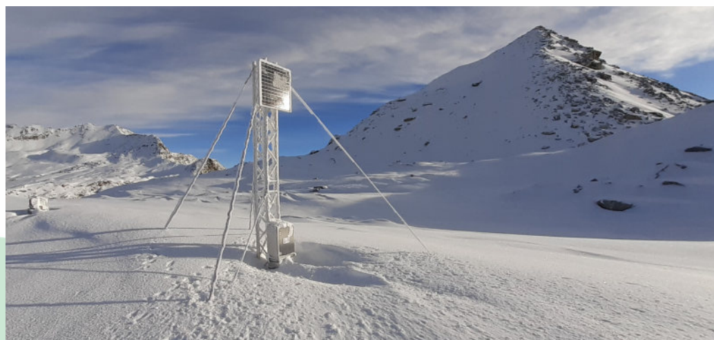
Fig. 29. Mt. Moro Pass permafrost monitoring station, 2870 m a.s.l., Municipality of Macugnaga, VB. In this site, new calibrated datalogger and thermistor chain have been installed in borehole 30 m deep since 2018, in order to evaluate the climate change effect on permafrost in Monte Rosa area. Photo: Luca Paro.
