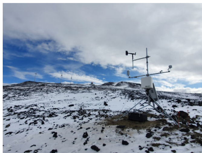
Fig. 39. The new Scott Base soil climate station, Crater Hill and the wind farm in the background.
