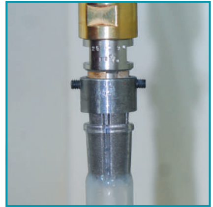
Grinding steps are performed by diamond reamers assuring best results with highest precision.
