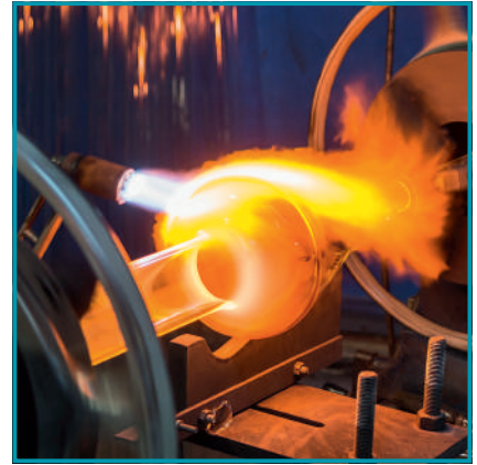
Glass tubes are blown by highly skilled blowers to ensure the uniform wall thickness, exact dimensions according to DIN standards.
