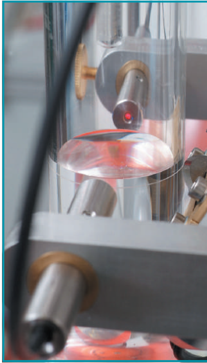
Meniscus is determined automatically at the exact lowest level by a laser beam.
