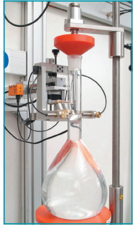
Filling the blank products with water is done automatically by the calibration machines.
