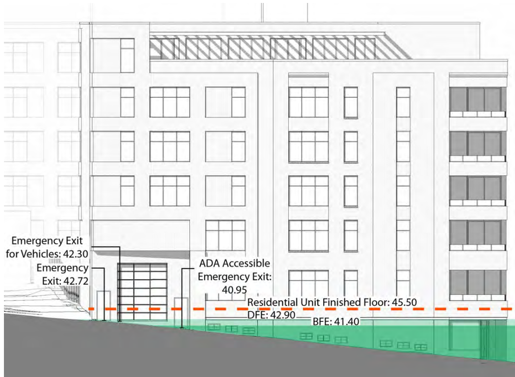
Figure 2: Elevation view of west building (per CBP Architects 3/11/24 plans) with key flood and building elevations
