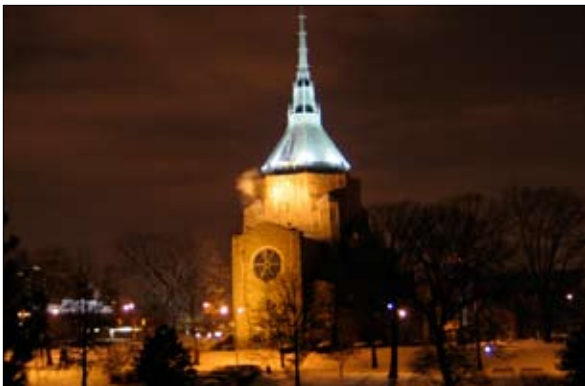
This Cleveland church spire has been creatively lighted in a cool metal halide contrasted against warmer high pressure sodium vapor light. Areas adjacent to the building are well lit with reflected architectural light.
