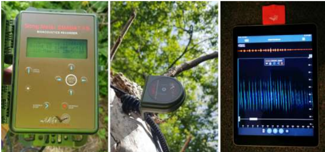
Figure A 18 Bat detectors - SM4 static recorder and microphone, Echometer handheld detector
