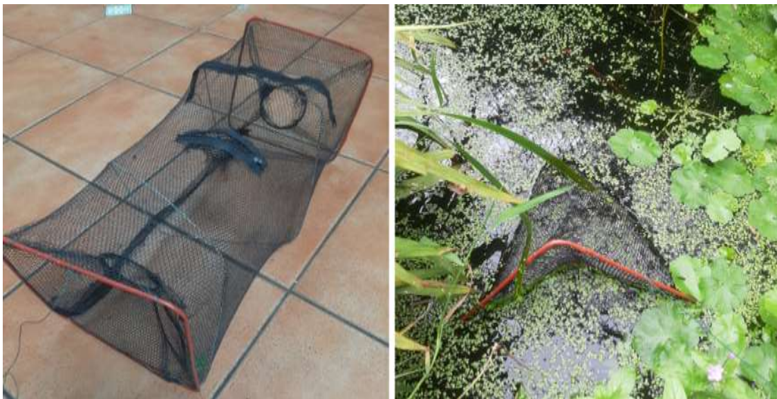
Figure A 29 Fish trap, out of water and submerged, used in smooth newt and common frog surveys. Photos: Collie Ennis.
