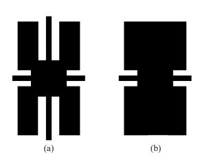
Figure 5: Modification of PBG cell, (a) The classical cell structure, (b) Modified PBG cell structure.
