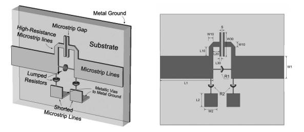
Figure 4: Improved equalizer structure with parameter denition.
