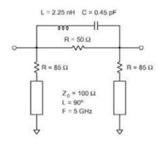
Figure 2: The traditional equalizer circuit.
