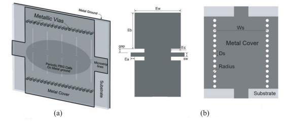
Figure 7: The proposed PBG structure and the parameter definition, (a) Modified PBG structure, (b) Congurations for PBG cell and the SIW with their geometric parameters.
