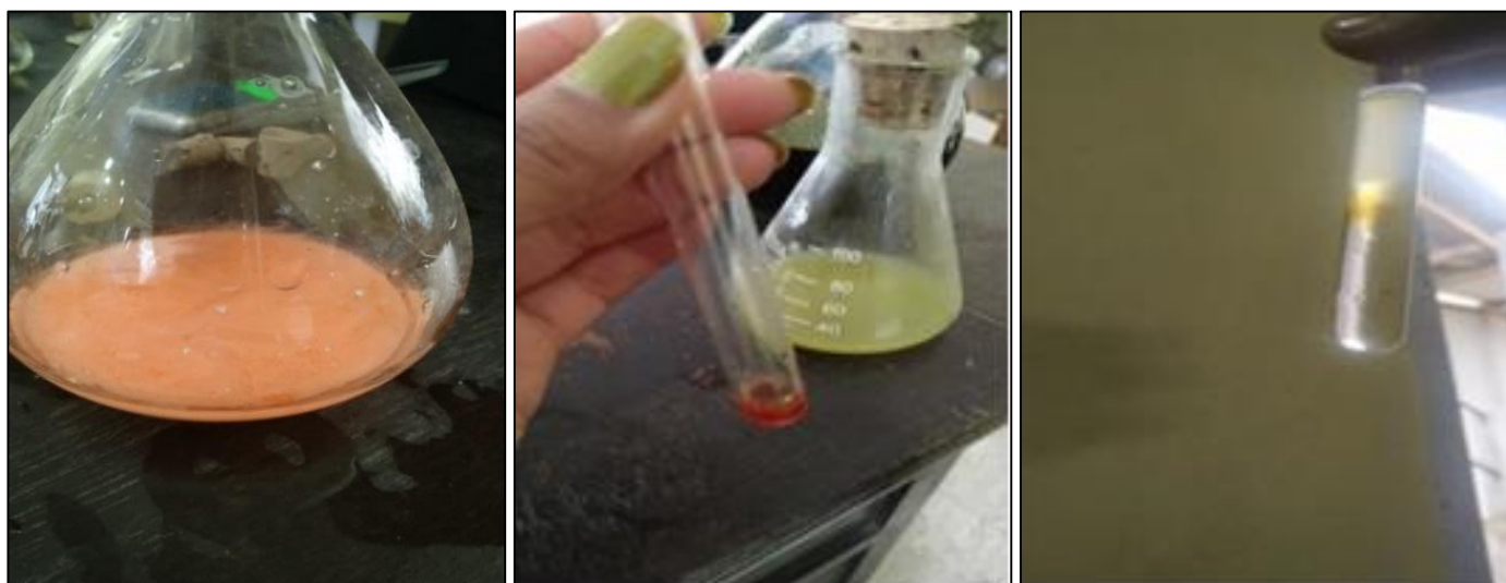
Fig 5(a): Crude extract of Gynocardia odorata fruit (b) Test showing the presence of alkaloid ( Dragendroffs test) and terpenoid extracted from hexane solvent
