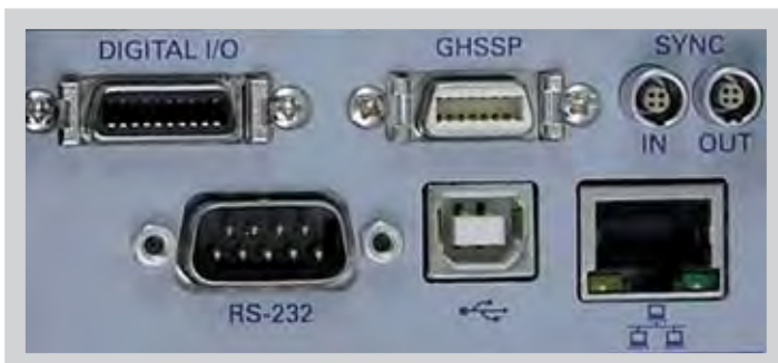
PI controllers are available with a number of different interfaces for highest flexibility. In addition to the modern Ethernet (TCP/IP) and USB, many industrial customers still appreciate the robust RS-232 protocol
