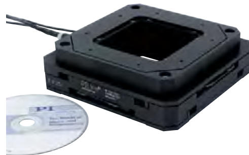
M-686 open-frame stage with P-541.2DD piezo scanner on top, providing a resolution of 0.1 nm and a scanning range of 30 x 30 \mu\text{m} . The system height of the combination with the P-541 XY (or Z) piezo scanner is only 48 mm
