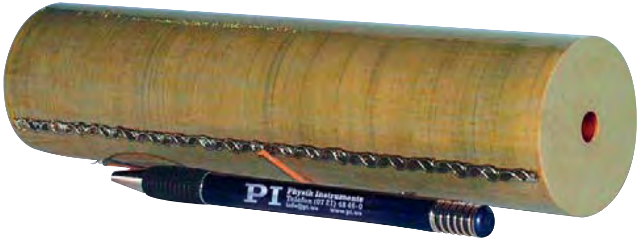
Custom PICA™ Thru piezo actuator with 56 mm outside diameter, 8 mm inner diameter, 250 \mu\text{m} displacement. Pen for size comparison
