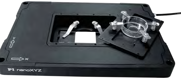
PI nano™ series nanopositioning stages feature a very low profile of 20 mm (0.8), a large aperture for 3 x 1" slides and deliver highly accurate motion with sub-nanometer resolution in up to 3 axes. Slide / petri dish holders optional
