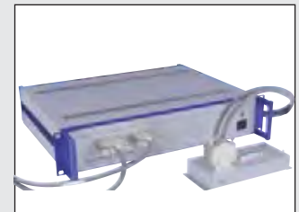
Fig. 11: Digital sensor-signal transmission (DST) allows a distance up to 15 m between positioning unit and controller, here an E-710 multi-axis digital piezo controller
