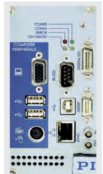
The E-712 provides RS-232, USB and RS-232 as standard interfaces. Additionally, digital I/O lines and optional analog interfaces or a real-time PIO are available.
