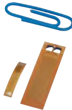
Fig. 13. Strain gauge sensors. Paper clip for size comparison
