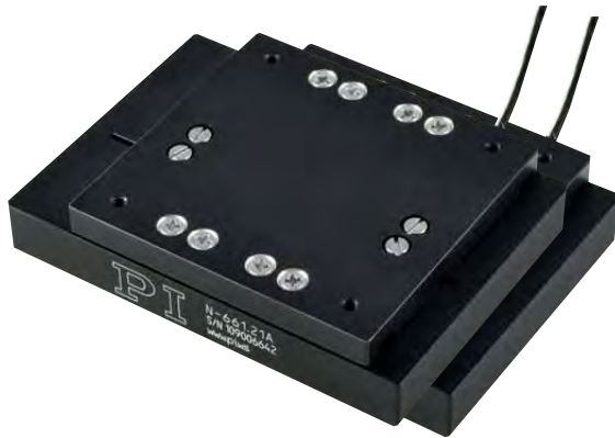
The N-661 miniature linear stage integrates a PiezoWalk® NEXACT® linear motor combined with a high-resolution linear encoder. It provides 20 mm travel and resolution down to the nanometer range.
