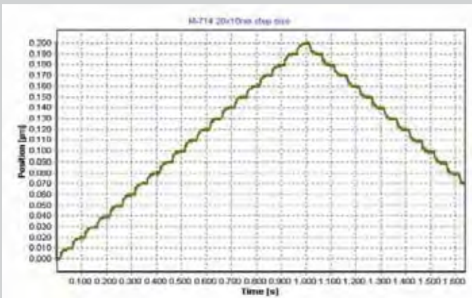
10 nm steps of an M-714 stage, as commanded by a C-702 digital controller and measured by an interferometer
