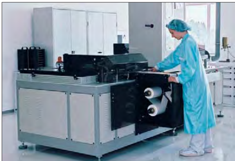
Equipment for fully automated screen printing of electrodes on piezoelectric and dielectric ceramics.
