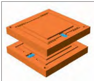
Design principle of a stacked XY piezo stage (serial kinematics).
