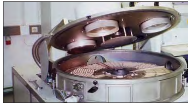
Sputtering facility at PI Ceramic
