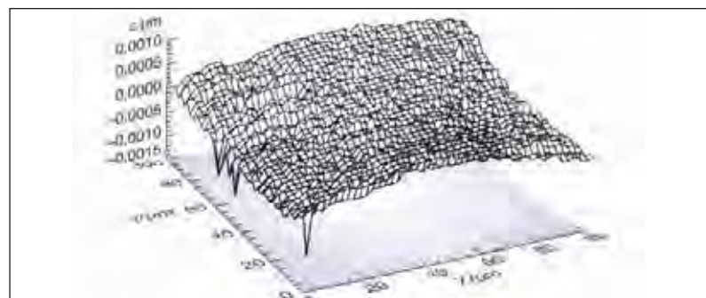
Flatness of an active-trajectory-controlled nanopositioning stage over 100 x 100 µm scanning range is about 1 nm
