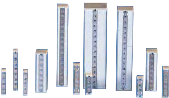
Fig. 39 a. PICMA ® actuators are made with ceramic-only insulation and can dispense with any polymer coating. Result No measurable outgassing, insensitive to atmospheric humidity and a wider operating temperature range
