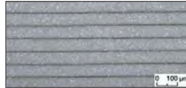
Piezoceramic layers in a monolithic actuator (LVPZT).
