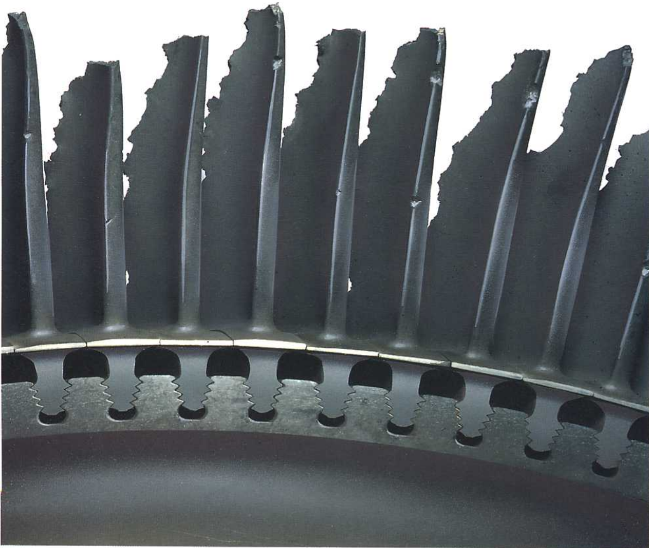
Fig. 24-9 Overheated turbine blades.
