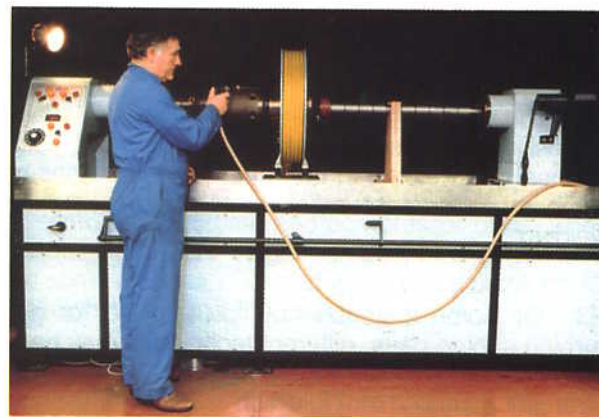
Fig. 25-3 Magnetic crack testing.
