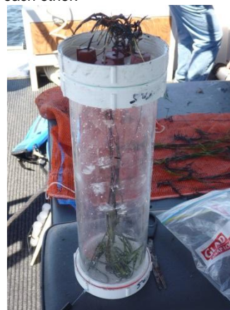
Close up of the top chamber with the two way screw cap. The leaves of the seagrass fronds are threaded through the rubber bung in such a manner that the leaves remain in the Perspex chamber and the rhizomes in the bottom.
