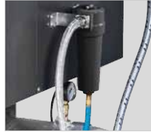
· Microfilter installed as filter upstream of compressed air take-off for separating condensate and dirt with particle sizes of up to 25 µm · Compressed air quality as per ISO 8573-1
