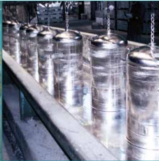
Hot-dip galvanisation for a long service life
