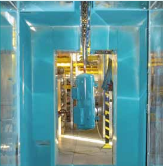
Environmentally-friendly powder coating plant
