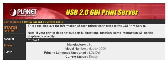
This page lists the information and the status of the printer connected to the GDI Print Server USB port. The printer information includes manufacturer, model number and the supported printing language. The status of the printer include "Ready", "Off Line" or "Paper Out".
