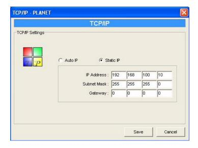
Double Click "TCP/IP" icon and the TCP/IP configuration window will pop-up. You can configure the GDI Print Server to automatically get IP from DHCP
