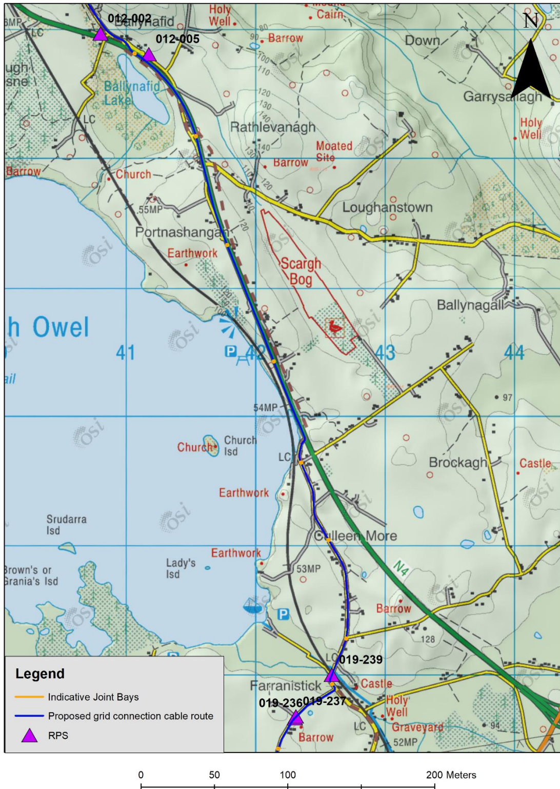
Figure 13-28: RPS structures within 100m of the proposed Grid Connection Route at Ballynafid and Farranistick.
