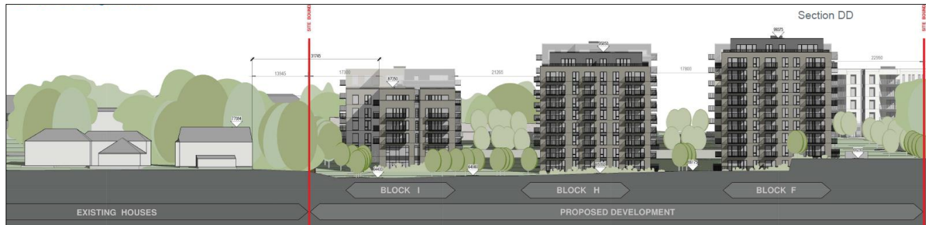
Figure 10.19 Section-elevation showing the step down in height towards the west site boundary and the nearest houses in Brennanstown Vale
