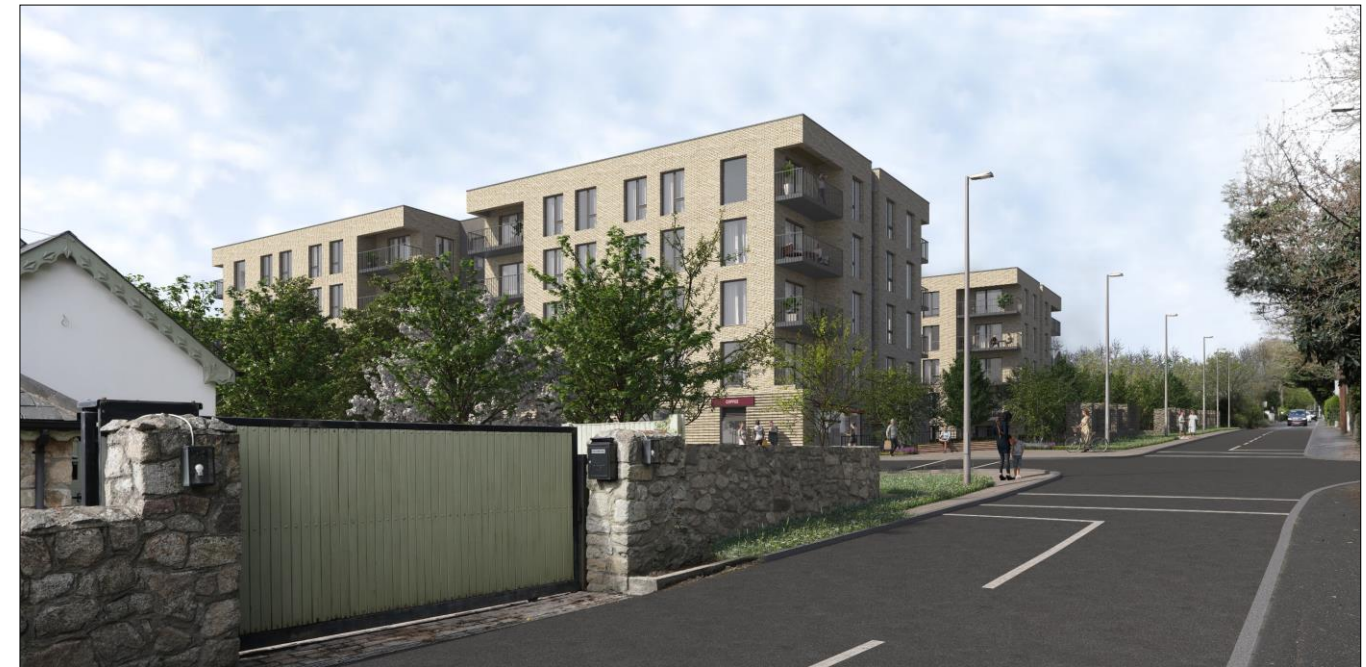
Figure 10.15 Photomontage showing the set-back, permeable built frontage to Brennanstown Road, the separation distance of Block C-D from the nearest house to the east, and the wide green strip including trees in front of the buildings to soften their presence on the road. Note the central vertical recess in the long east elevation and the corner recessed balconies to articulate the massing.
