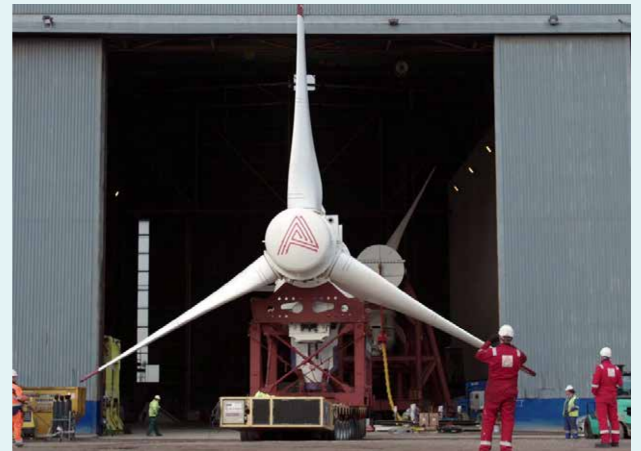
The AR1500 tidal turbine (Source: SAE Renewables)
