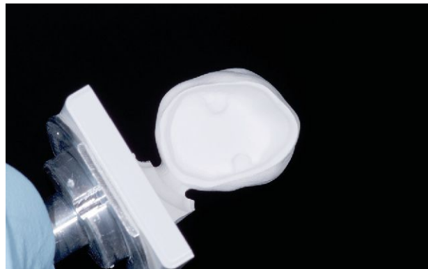
Fig. 3: Milled KATANA STML restoration on super-fast mill setting in CEREC® Primemill without chipping
