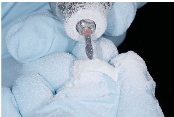
Fig. 4: Sprue removal using carbide burs at 10,000 rpm in a lab handpiece
