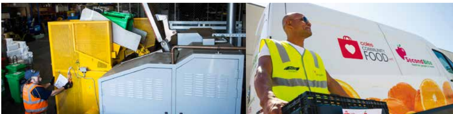
This 1200lt GaiaRecycle machine processes 8.4 tonnes of organic waste a week
