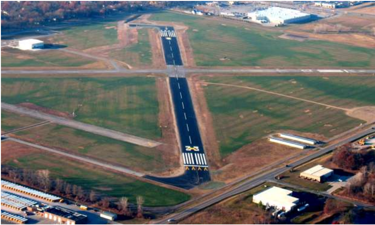
Figure 2-1 Markings for a Temporarily Closed Runway
