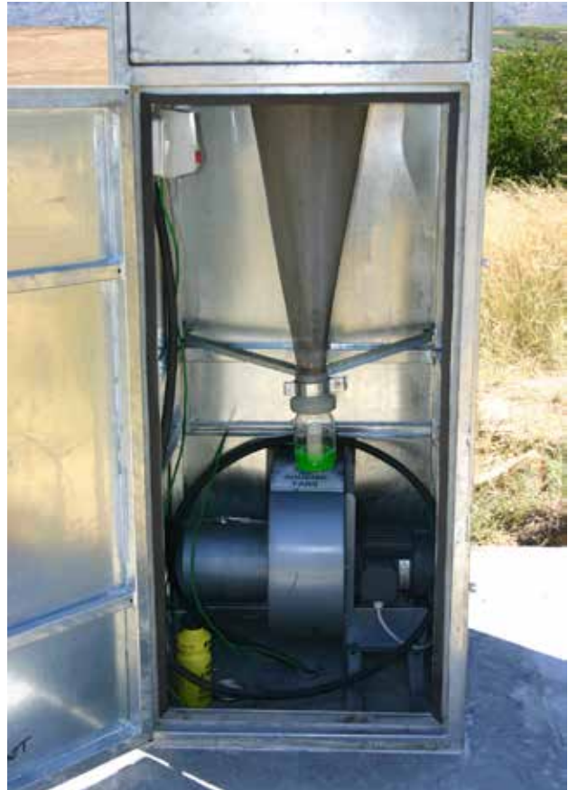
Suction trap on the inside showing the fan and bottle with preservative in which aphids collected
