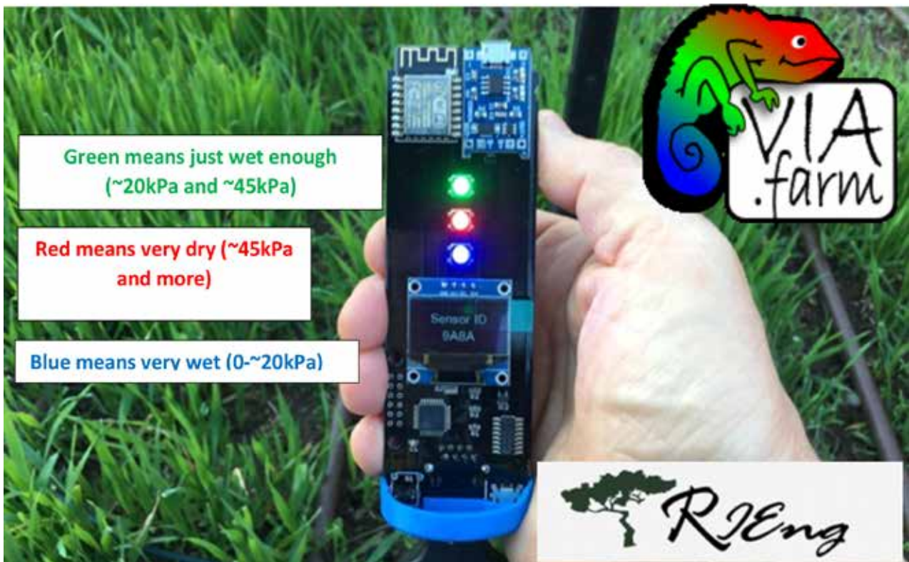
Figure 3: Chameleon field reader and each colours' meaning
