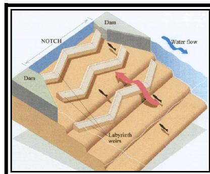
A conceptual design of the notch and "W" shaped weirs of the new fishway at Little Falls. The three weirs slow the water down through the 28' wide notch and provide rest areas for migrating fish.
