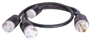
CBL149 Splitter Cable L21-30R to (3) L5-30R (4 ft/2 ft/1 ft)
