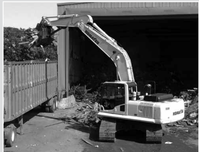
Komatsu's new PC200LC-8 Waste Spec Arrangement is built for the rigors of waste handling in transfer stations, landfills and construction and demolition debris applications. Features such as wide core coolers keep the machine temperature down for better production even in the most severe environments.
