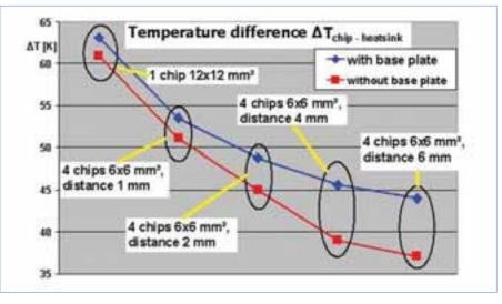
Figure 3. Chip temperature in modules with baseplate and modules based on SKiiP technology as a function of the chip clearance (simulated with 2W/mm<sup>2</sup> power loss).
