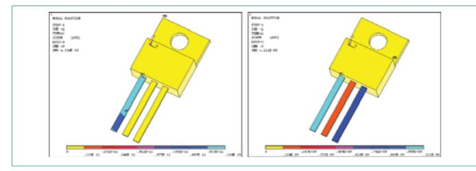
Figure 6a. Normal VS Contamination current density; 9.39E-12A/mm2 (normal) Figure 6b. Normal VS Contamination current density; 1.04E-9A/mm2 (Contamination at gate connection)
