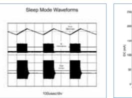
Figure 2. Typical switching and output voltage waveforms in sleep mode.
