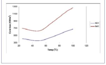
Figure 2. Core loss temperature diagram for N41 and N51.
