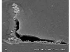
Figure 5. Passivation crack after KOH etching in Igss high sample.
