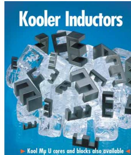
Inductors made from Magnetics'® Kool Mu® E cores run cooler than those made with gapped ferrite cores. Eddy currents, caused by the fringing flux across the discrete air gaps of a gapped ferrite, can lead to excessive heat due to heavy copper losses. The distributed air gaps inherent in Kool My can provide a much cooler inductor.
