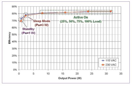
Figure 5. Efficiency vs. Output Power PeakSwitch Design Example.
