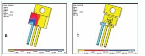
Figure 2a. Potential distribution of external package. Figure 2b. Potential distribution of internal package.
