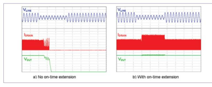
Figure 3. Impact of Adaptive On-time Extension.
