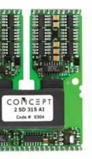
Driver stage for a gate current up to ±15A per channel, stabilized by large ceramic capacitors
