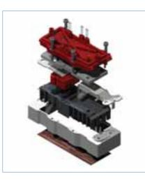
Figure 2. Exploded view of the IGBT halfbridge.
