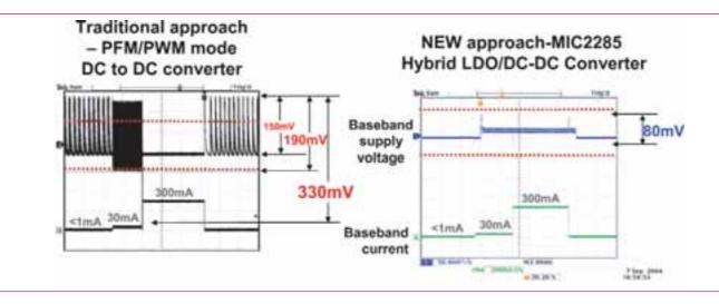
Figure 4. Comparison of Load Profiles for Industry Standard Buck Regulator Using a PFM Mode Light Load Scheme Compared to the MIC2285 Offering a LDO Mode in Light Load.
