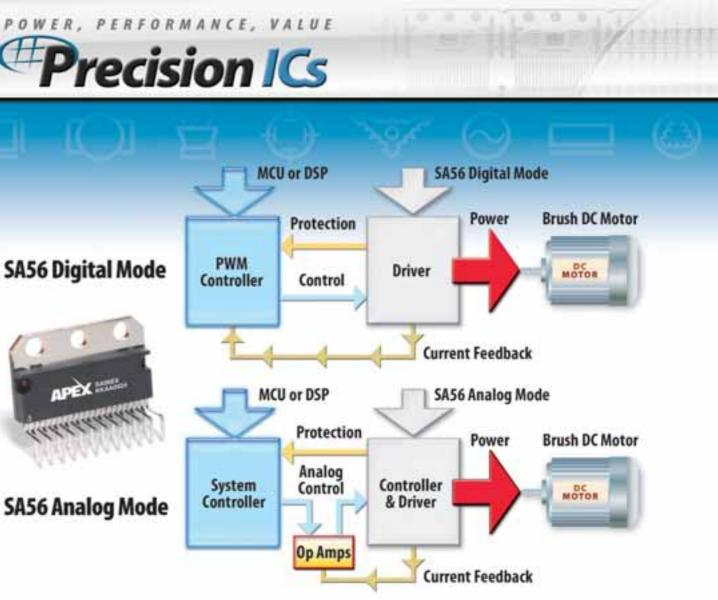
Industry's first 5A monolithic PWM amplifier works with digital or analog control to drive bi-directional DC motors up to 1/3HP on 55V supplies.
