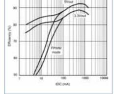
Figure 5. The resulting efficiency measurement shows a significant improvement in the efficiency for currents below 50mA load.
