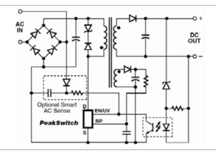
Figure 1. Typical Application Schematic with PeakSwitch
