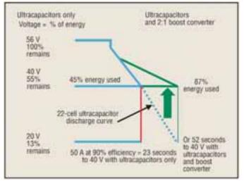
Figure 2. Discharge curves for ultracapacitors with and without power electronics.
