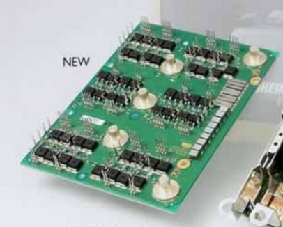
POWER BOARD ASSEMBLY (ACTUAL) (48) FETs (9) Low profile capacitors (5) Low profile bus bors Total Wt. 370.6 g
