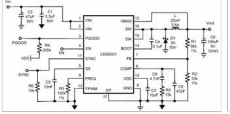
Figure 4. Typical application circuit with the few required external components.
