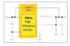
Figure 3. MIC2285 Conceptual Internal Block Diagram That Shows a LDO in Parallel with 8MHz PWM Buck Regulator.
