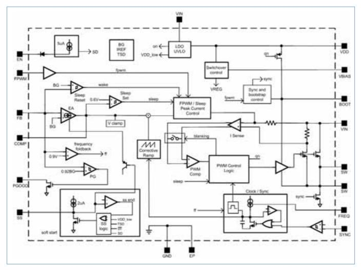
Figure 1. Internal block diagram, shows all of the typical elements of the LM26001
