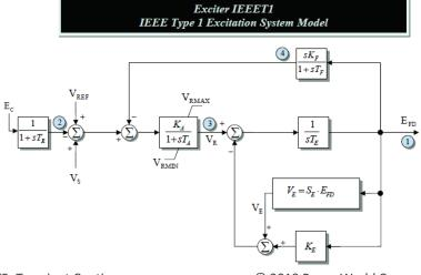
The input to the exciter,  $E_c$ , is usually the terminal voltage. The output,  $E_{FD}$ , is the machine field voltage.
