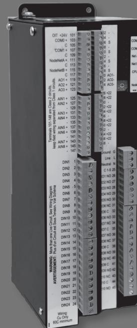
FSC - Flexible System Controller terminal blocks
