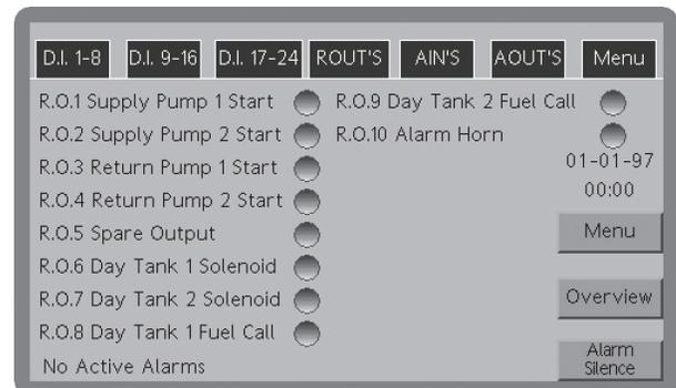
Typical relay output screen helps troubleshoot controlled devices.
