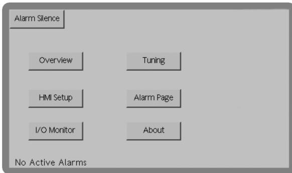
Typical main menu screen used to navigate between overview, setup, alarm, and other screens.
