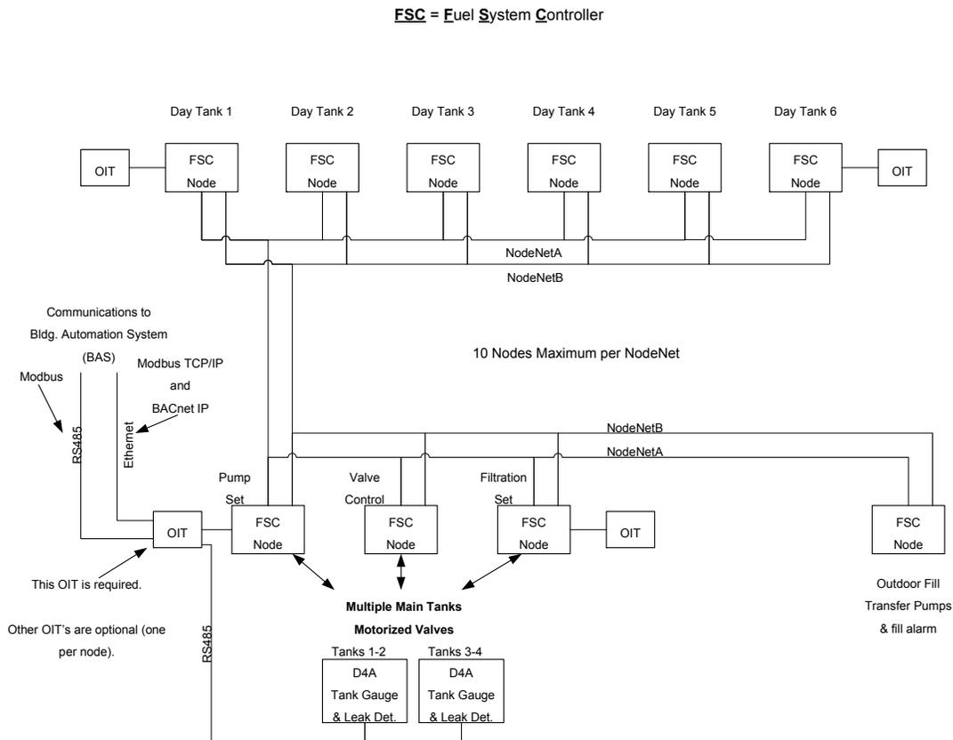
Ten FSC controllers in an emergency generator application with six day tanks, two bulk storage tanks, duplex pump set, filtration system, and interface to a building automation system.
