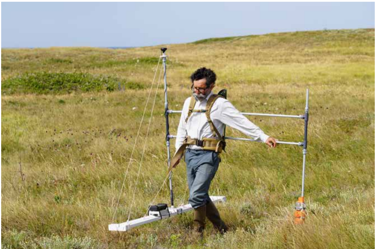
Fig. 9 – Implementation of the GEM 2 conductivity meter (Geophex, Ltd). The GNSS antenna is placed at the end of a mast to maintain a constant relative position between the measurement and the determination of its position. The carrying device, made of neutral materials (plastic and fibreglass tube), helps to keep the conductivity meter horizontal as the operator is walking (photo P. Arias).
