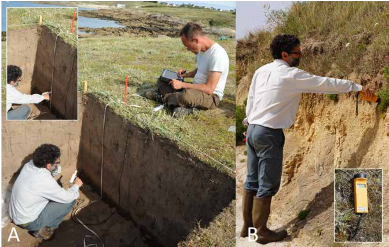
Fig. 4 – Implementation of susceptibility meters by contact measurement. A: MS2K (Bartington) computer controlled with its MS3 electronics. The advantage of this probe is its small diameter, about 2.5 cm, but the downside is its shallow depth of investigation, of about 1 cm. B: KT9 (Exploranium). The advantage of this instrument is its speed of measurement. The probe diameter of about 6 cm provides a detection depth of 2 to 3 cm. A measurement in air is necessary before and after the measurement carried out in contact with the measured surface.
