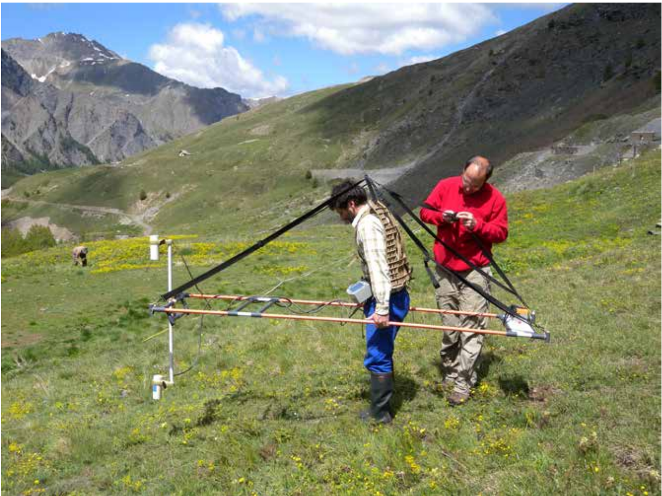
Fig. 2 – Sensor arrangement of a G858 Geometrics optically pumped magnetometer in a gradiometer (photo L. Carozza).
