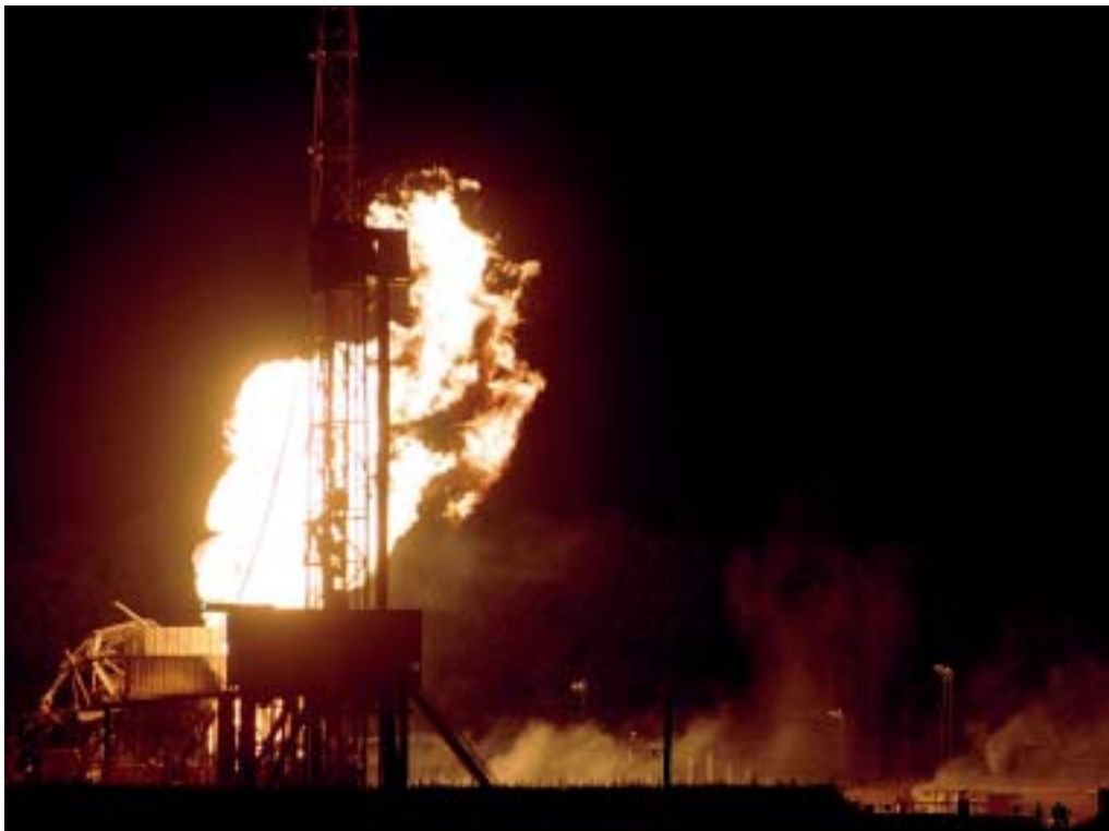
Blowout: The huge cloud of flaming gas could be seen from miles away.
