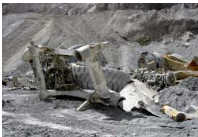
HDTs were at the mercy of the falling material. One of the colossal trucks – 5 m high and more than 10 m long – lies in ruins.
