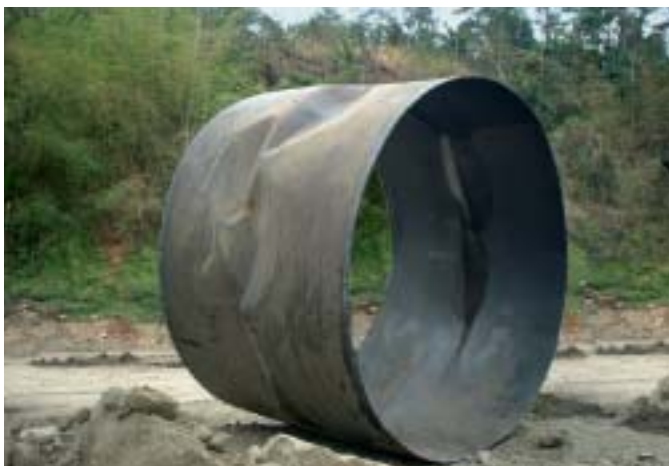
Pipe segment distinctly deformed, unable to support the pressure of the backfill material.
