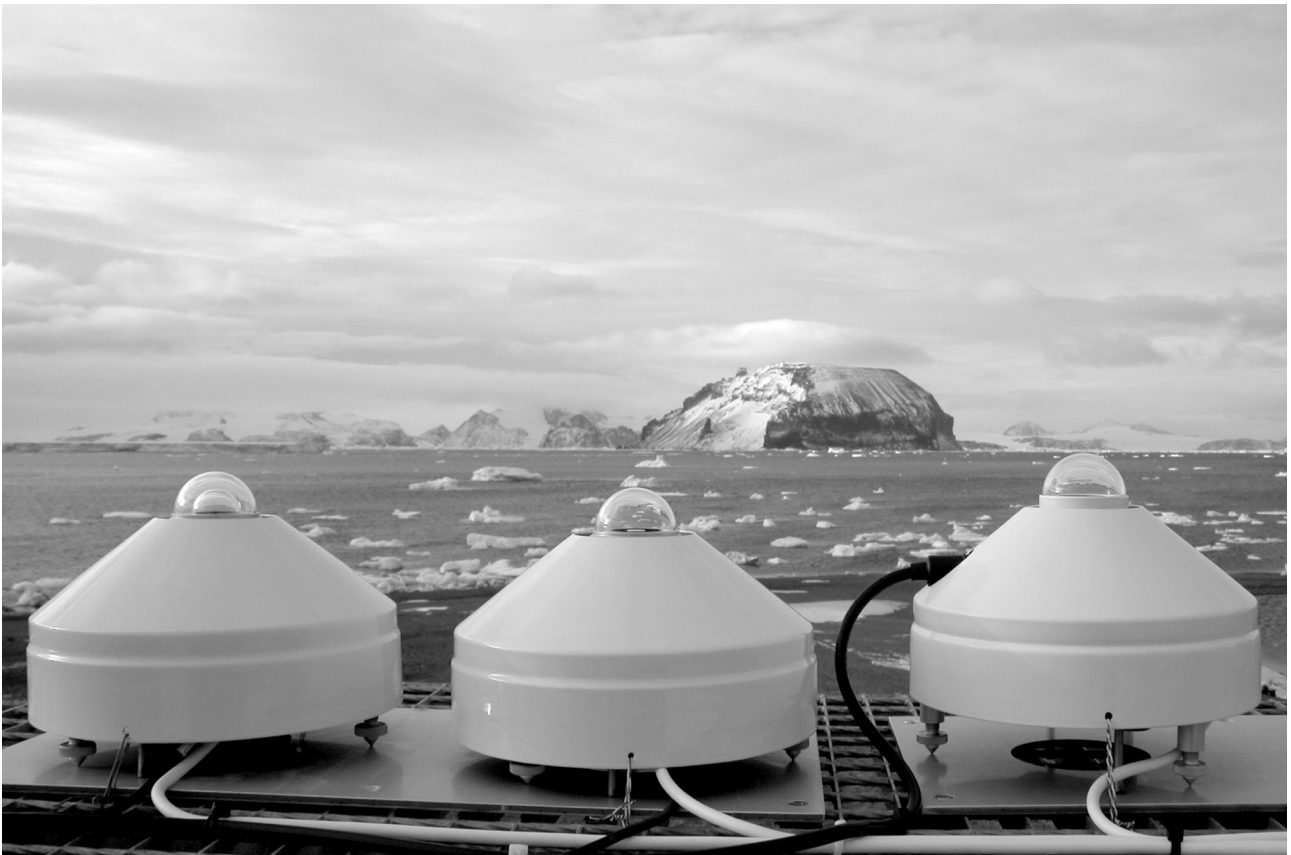
Fig. 1 The set of radiometers equipped with the Kipp-Zonen ventilation units installed on a special platform at the J.G. Mendel Station (photo K. Láška).
