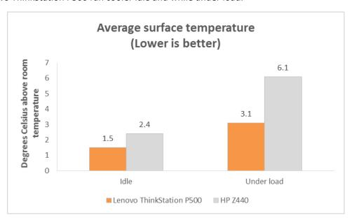
Figure 2: When idle and under load, the **Lenovo ThinkStation** P500 ran cooler than the HP workstation.
