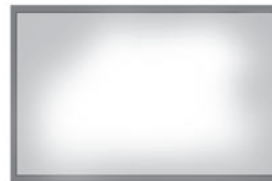
Without DUE: uneven brightness distribution
