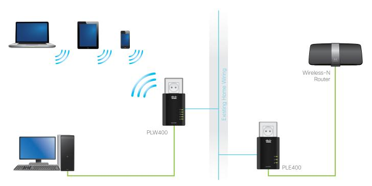
By simply plugging in the two Powerline adapters to your home network, a new internet connection is created for ethernet enabled devices
