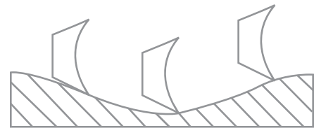
COFA blade geometry cutting uneven surface.
