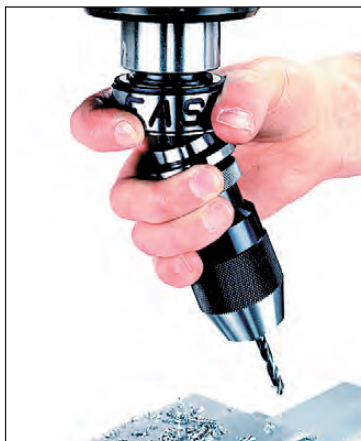
3. Removing drill chuck holder with one hand.
