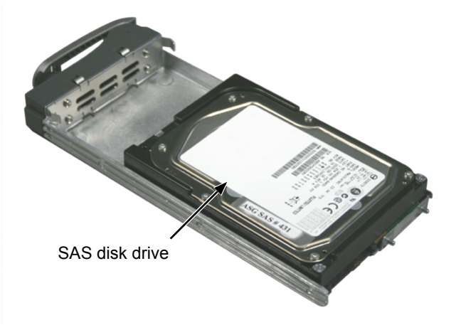
Figure 10. SAS drive mounted in a drive carrier
