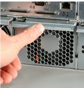
Figure 12. Locking the cooling unit handle (left: E610f/s, right: E310f/s)
