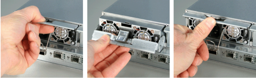
Figure 2. Replacing an E310f/s power supply
