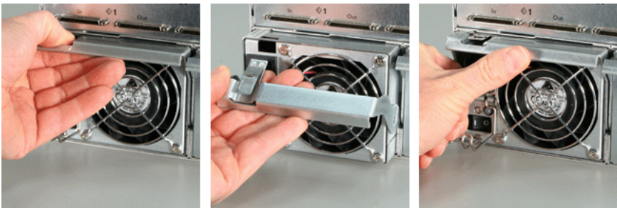
Figure 1. Replacing an E610f/s power supply
