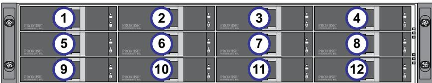
Install all of the drive carriers into the VessJBOD enclosure to ensure proper airflow, even if you do not populate all the carriers with disk drives.
