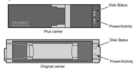
If there is a disk drive in the carrier, the Power/Activity LED displays green. If not, the Power/Activity LED remains dark. The Power/Activity LED flashes during drive activity.
