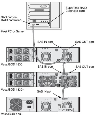
Figure 7. Data connections with SuperTrak
