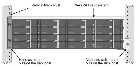
Figure 1. A 16-bay VessJBOD mounted in a rack with the available rails
