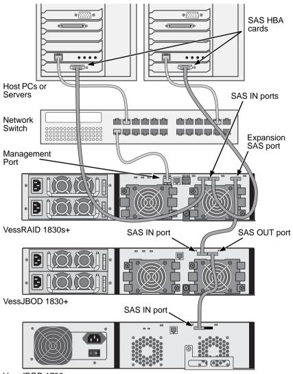
Figure 6. Data and management connections with VessRAID
