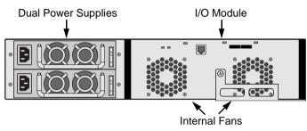
Figure 5. VessJBOD 1830+ rear view
