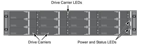
Figure 3. VessJBOD 1730 rear view
