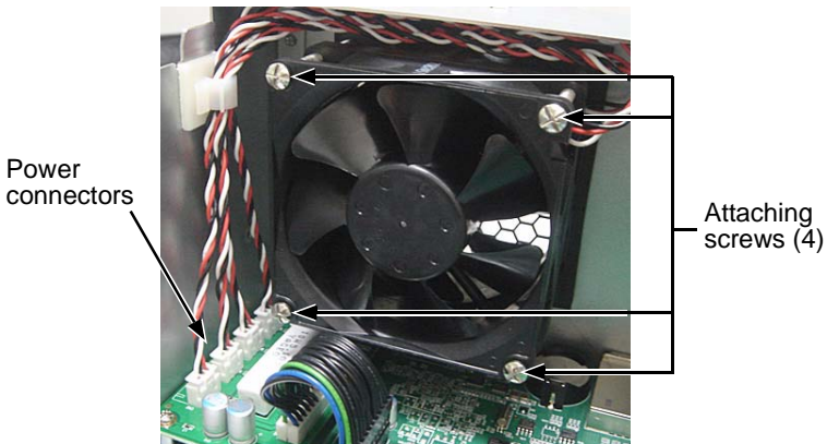
Figure 4. I/O module cooling fan. 3U model shown
