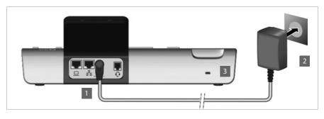
Connect the power adapter to the port on the rear of the phone.
