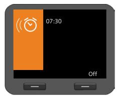
A wake-up call is signalled on the display and the selected ringer also rings for 60 seconds.
