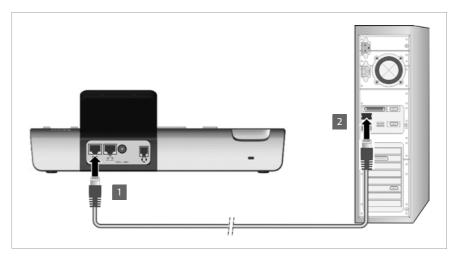
Connect an Ethernet cable to the left-hand LAN port on the rear of the phone.
