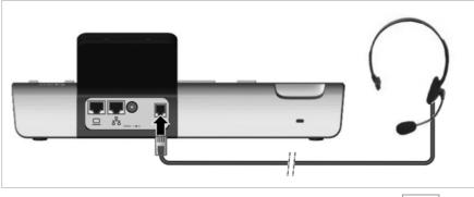
Connect the cable for the headset to the RJ9 connector on the phone.
