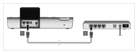
Attach one end of the Ethernet cable supplied to the right-hand LAN port on the rear of the phone.
