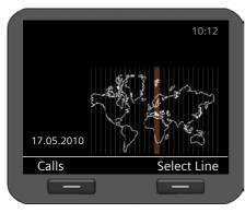
When setting the **Time Zone**, a map of the world showing the time zones appears on the screen. The current setting is highlighted.
