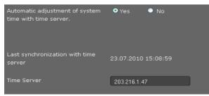
• Enter the IP address for the required time server in the Time Server field.
