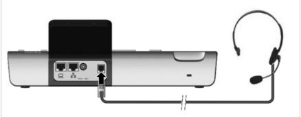
▶ Connect the cable for the headset to the RJ9 connector on the phone.
