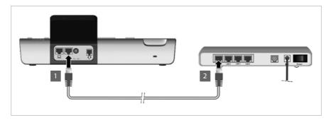
1 Attach one end of the Ethernet cable supplied to the right-hand LAN port on the rear of the phone.
