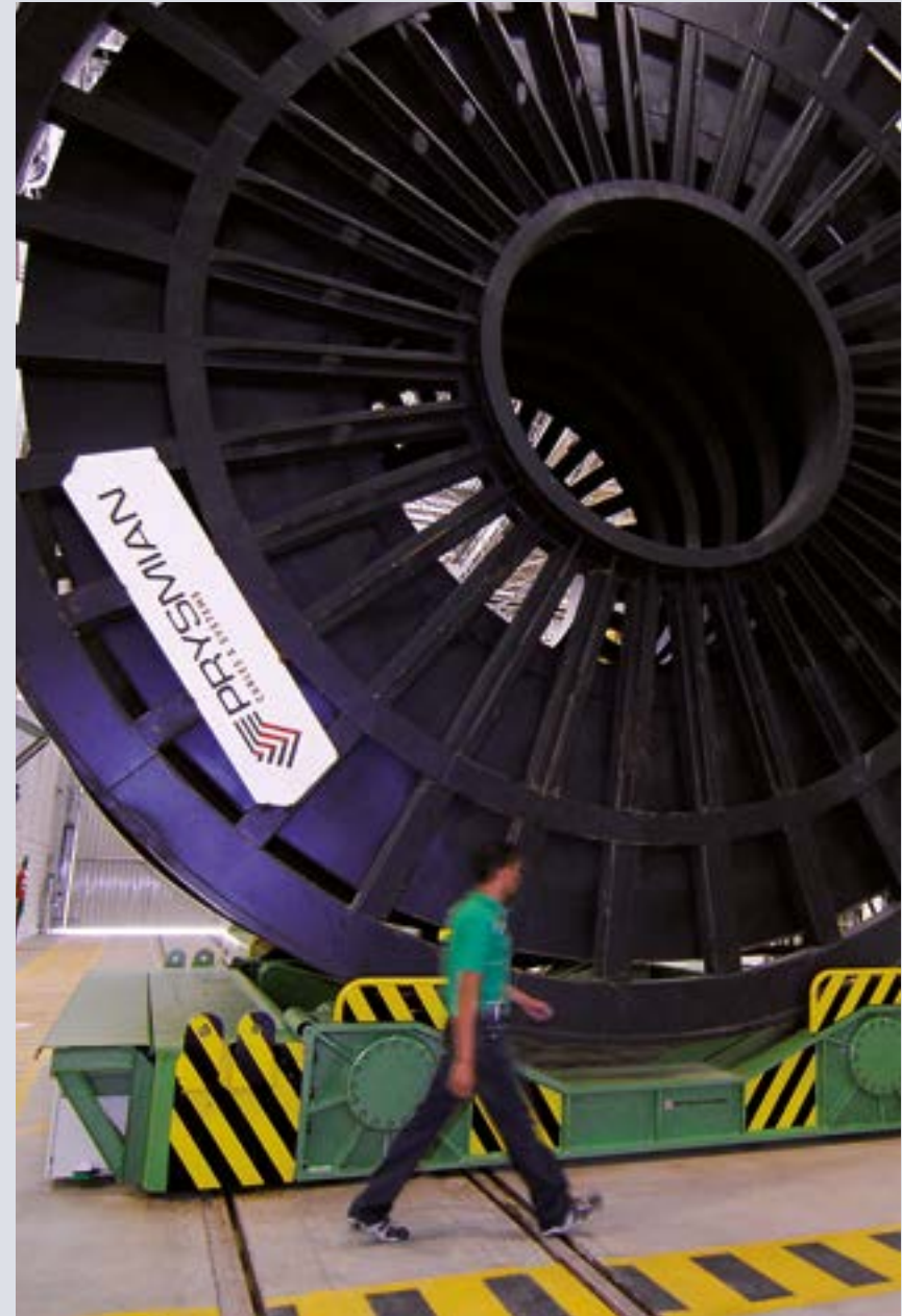
Drum for umbilicals in the Vila Velha plant, Brasil.
