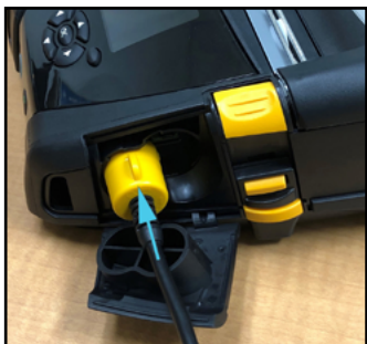
1. Insert connector in communications port.
