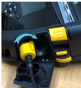
2. Rotate locking cap clockwise to secure.
