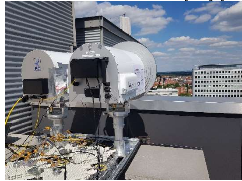
FIGURE 15. 300 GHz ThoR link connecting two buildings at the campus of TU Braunschweig.
