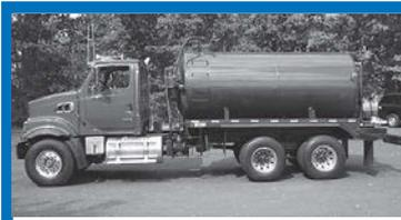
**2008 Sterling LT9500:** Mercedes 6-cylinder (450hp). Fuller 8LL. Aluminum wheels, A/C, power locks & windows, 66k GVW. Dickirson Septic Truck, 3,000 gallon, steel tank. Masport PTO-drive pump. 149,278 miles. Stock# 8405 .... \$79,500
