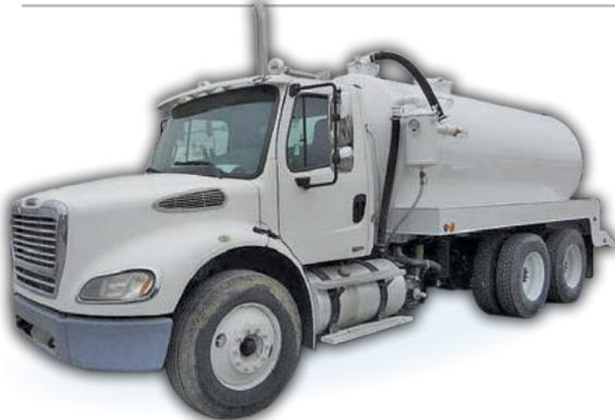
**2007 Freightliner M2-112**, Cat 335 HP, 10 spd, jakes, 14,700 fronts, double framed, **new** 3360 gallon steel vac tank, **new** Masport 400 Vac pump.
