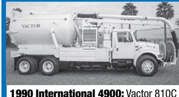
**1990 International 4900:** Vactor 810C combo sewer cleaner, 60gpm pump, 15-yard debris tank, 1,000-gallon water tank, 2-stage fan. Stock# 3317656. .... \$59,500
