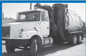
**1994 Cusco/Volvo Mastervac Wet Dry** DOT/312 3,000-gallon carbon steel vacuum truck. 27' Hibon blower with Moro off-loading pump. CAT engine with Fuller transmission.
