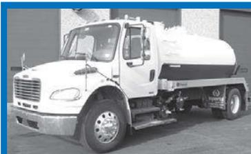
**2007 Freightliner M2** with new 2,500-gallon Imperial tank, Masport 350cfm, 260hp, Allison automatic, air ride cab & suspension, ATC traction control. Stock# 373243.
