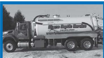
**2011 Navistar:** Automatic, 77,000 miles, like new. 4,000-gallon tank: 3,700 waste, 300 fresh water. Jetter system, 250' x 3/8" hose. Hoist hydraulically operated 3 stage. Full open rear door. Blower pump Robuschi RB-DV 65 950cfm. .... \$169,000
