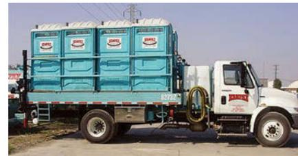
The rectangular vacuum tank from **Crescent Tank Mfg.** allows for the design of an all-in-one vacuum and restroom transport truck. Its low profile offers a lower center of gravity
