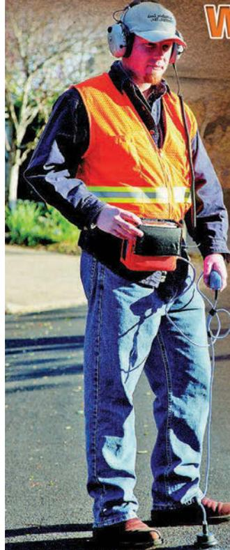
The LD-18 Digital Water Leak Detector uses patented technology to significantly reduce ambient noises from dogs barking, footsteps, people talking, etc. The digital amplifier samples the sounds every few tenths of a second, rejecting intermittent sounds instantly.
