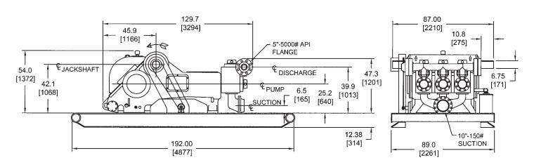
Note: All installations must contain a pressure relief valve in the discharge line near the pump.
